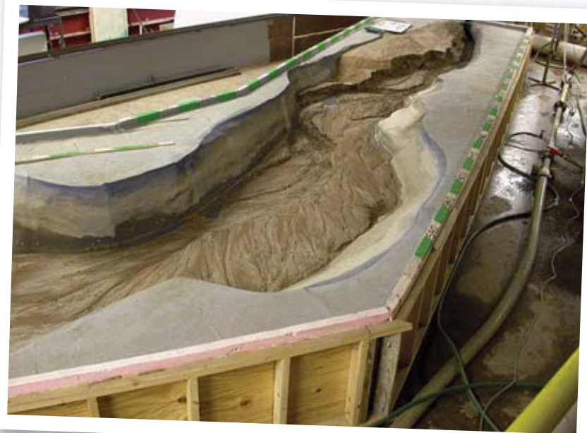
RIVER MODEL at the National Center for Earth-surface Dynamics in Minnesota provides scientists with a way to study how sediments move. This research can help experts plan what to do with the dirt and other material that accumulates behind dams.
